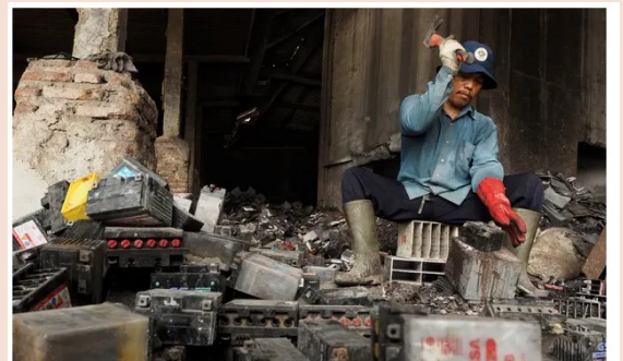
☞ A man in Tegal, Indonesia, uses a hammer to break up used lead-acid batteries by hand. Photograph: Larry C. Price/Pure Earth
